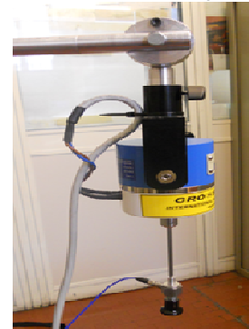
Figure 3. The piezoelectric load cell placed near the pushing tip.
